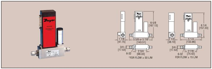
**Program, record, analyze, and control** flow rates of various gases with Series DMF Digital Mass Flow Controller. Controllers are designed with straight tube sensors with restrictor flow elements to ensure laminar gas flow for accurate and repeatable results. Series DMF are unaffected by temperature and pressure variations.
