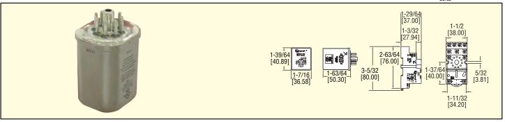
The Series 750H Hermetically Sealed Electromechanical Relay is designed to be used in Class I Division 2 hazardous area locations. Gold flashed contacts provide protection against oxidation in low current / voltage applications. 8-pin and 11-pin sockets are available to allow quick and easy installation for both surface and DIN rail mounting.
