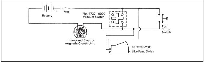
**REMOTE CONTROL** (When Engine Is Running): Install a pushbutton switch at one or more locations. Depress pushbutton for 2 seconds. If there is water in bilge, pump will operate until dry at which time vacuum switch will stop pump. If no water is in bilge, pump will stop when pushbutton is released.
